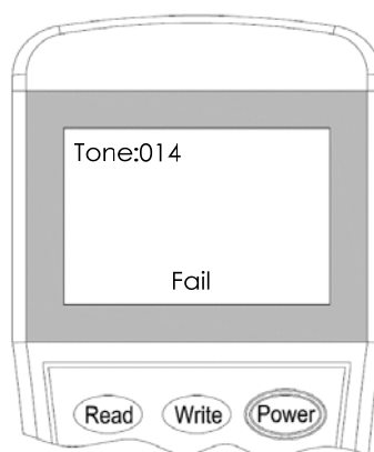
Fig.18 Fail to setting
