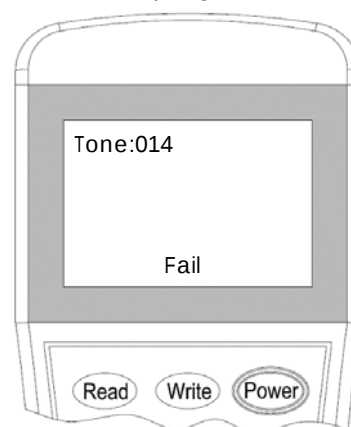
Fig.16 Fail to setting
